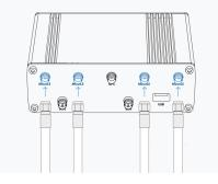
Power up the router by plugging in the 4-pin connector to the socket in the router
